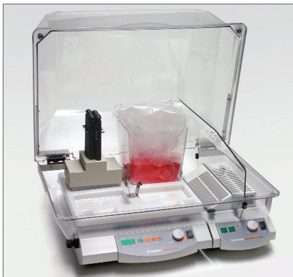
Fig. 1. The MAGDA Salmonella 24-hour plating assay involves enhanced enrichment lasting just 5½ hours, followed by immunomagnetic capture instead of a selective enrichment. Detection is done by familiar and approved plating.
